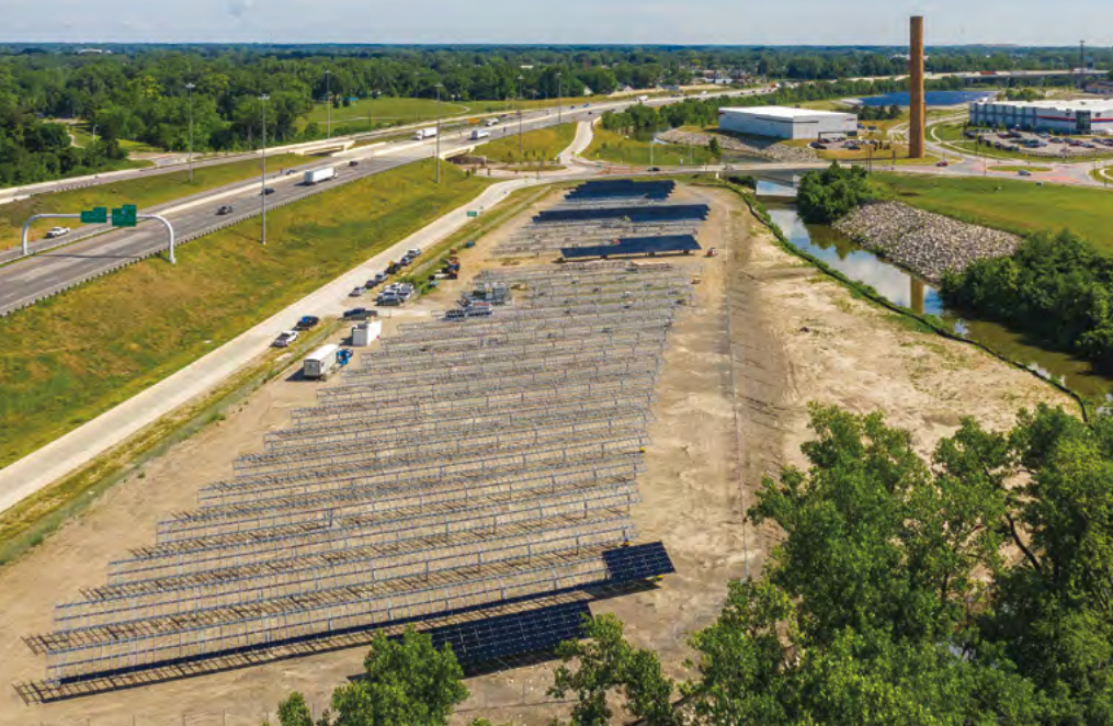
Community-based organizations in Toledo, Ohio, partnered to develop a 21,000-panel solar field on the site of a former Jeep manufacturing plant. Source: Toledo Aerial Media.
